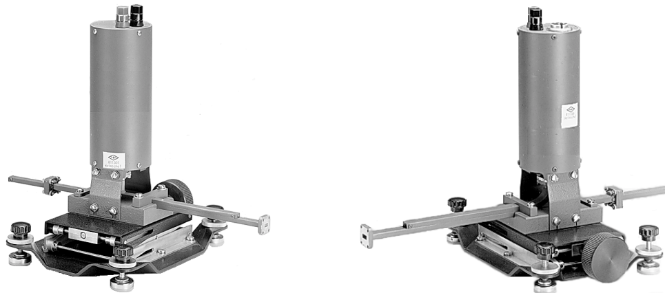
Figure 3-6 Waveguide Power Standards
